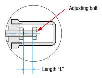
\*Set pressure: The pressure at which the relief valve starts to crack open (Cracking pressure) Refer to (B) in the operation chart described on the previous page.
