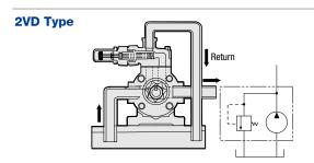
This is the same as the system above except for using a valve attached to Trochoid Pump 2HB directly.
