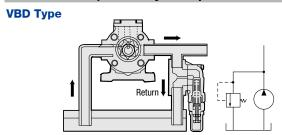
The valve is used as a pressure control valve for hydraulic oil or circulation oil lubricating system, which is installed with a sub plate.
